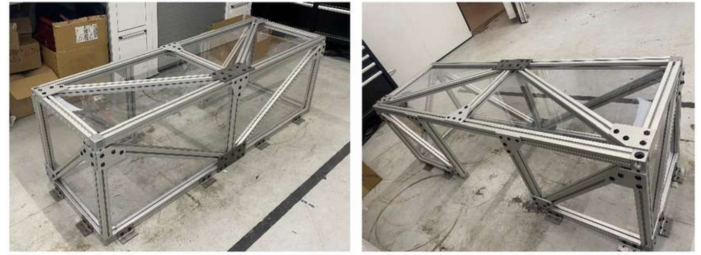
High-velocity projectile shield assembled by hand
