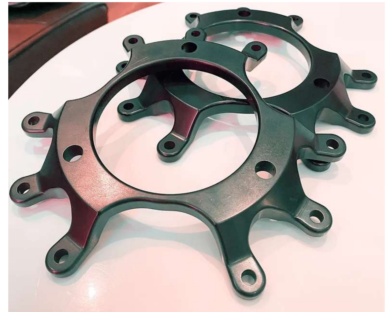
Final Product - Wheel centres made from 6061 aluminum
